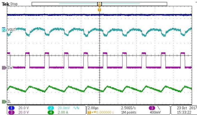
Figure 12. SW node waveform and Output Ripple
